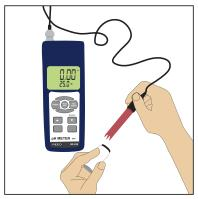
Remove the cap to take a reading of the aqueous ozone solution.
