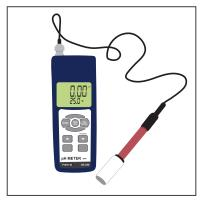
Inside the white cap on the end of the ORP probe, there is a sponge which can be kept moist with water.
