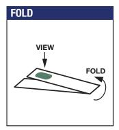
For best color matching, fold the white plastic handle of the test strip under the aperture so that it produces a white viewing background.
