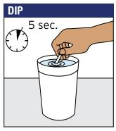
Dip ozone test strip into a 200mL room temperature water sample for 5 seconds with a constant, gentle back and forth motion (10 half strokes).
