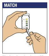
Match to the color chart at 30 seconds. Tersano SAO concentration is approved at **0.3ppm\***. A colour match at 0.5ppm exceeds the approved sanitation range testing.
