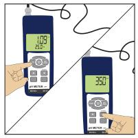
Push the **POWER** button to turn the meter on and the display will read the pH and temperature.
